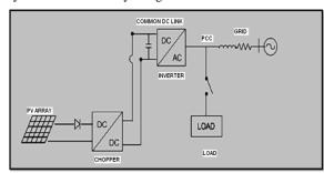
Fig: 1. Block diagram of PV grid connected system
