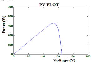
Fig: 10. P-V characteristics of the PV model
