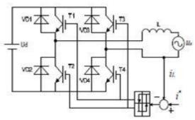
Fig: 7. Single-phase grid-connected inverter
