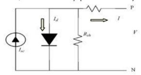
Fig: 3. Equivalent circuit of PV array
